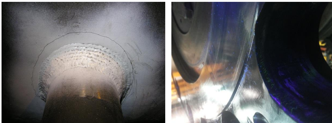
Figure 1.28 Examples of indications found using MT. Left: colour contrast ("black and white") applied at steam turbine part. Right: UV-fluorescence, applied at gas turbine disc.
