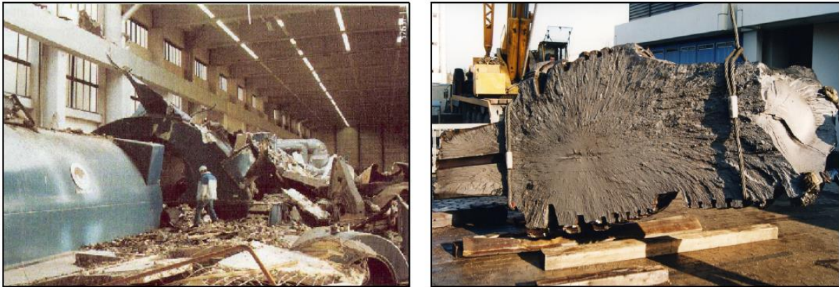
Figure 1.39 Low-pressure steam turbine failure
