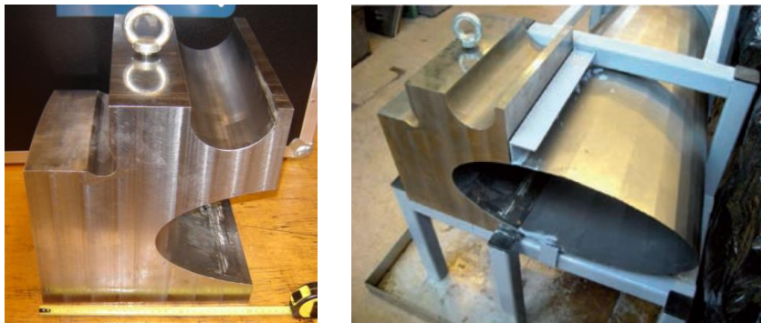
Figure 1.46 Left: test piece with spark eroded slots. Right: Mock up for testing handling of the manipulator
