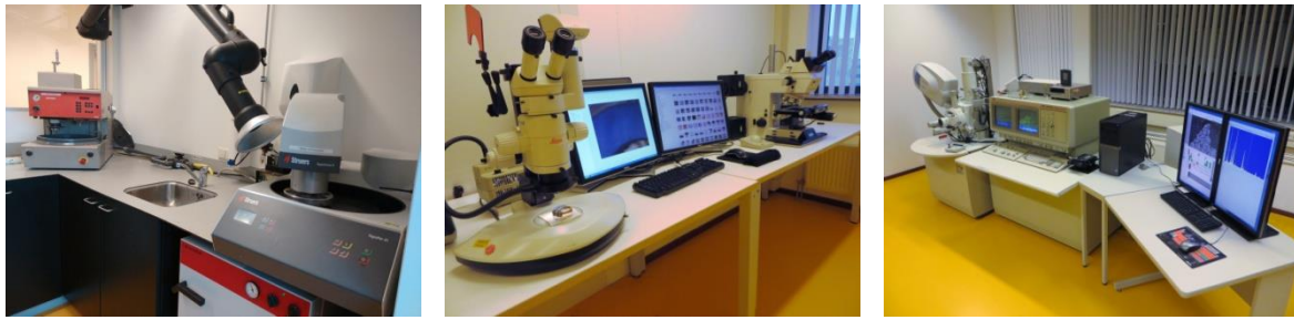
Figure 1.20 Left: sample preparation for microscopic investigation. Middle: stereo microscope ( magnification 8-100x) and metal microscope (magnification 25-1000x). Right: Scanning Electron Microscope (SEM).
