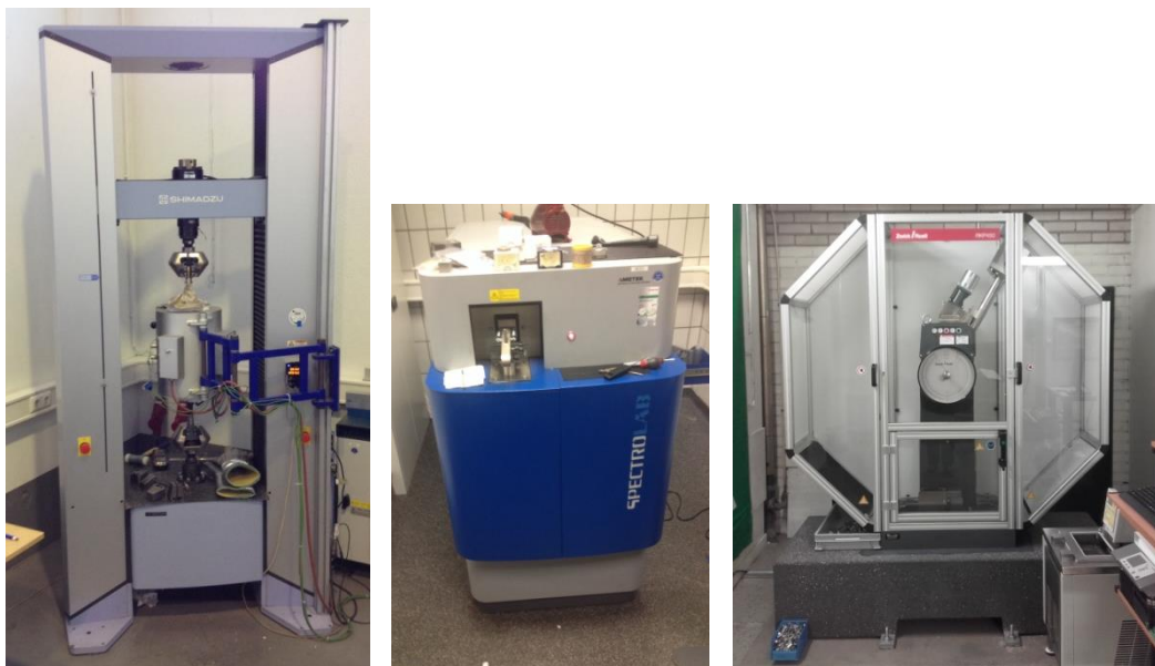
Figure 1.19 Left: universal testing machine (for tensile testing). Middle: Optical Emission Spectroscopy (OES) for accurate determination of metal composition. Right: Charpy Impact testing machine.
