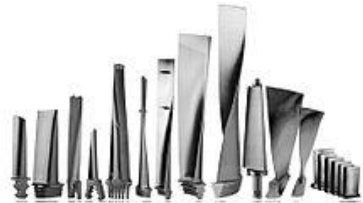
Figure 3.2 Different types of steam turbine blades
