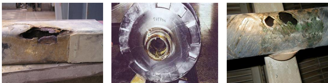
Figure 1.10 Typical damages observed in a FGD. Left: corroded steel beam with rubber; middle: impeller with radial cracks; right: holes in glass fibre reinforced plastic pipe.
