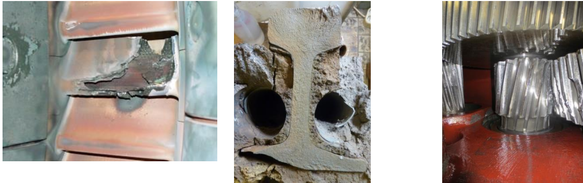
Figure 1.21 Left: first stage stationary gas turbine blade; middle: failed rail; right: broken bull and pinion gear
