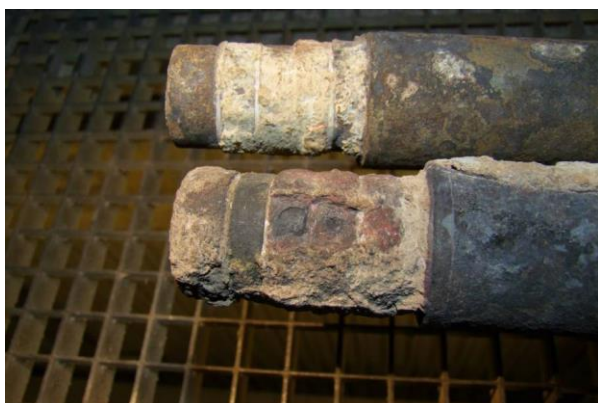
Figure 1.67 Tip of exposed corrosion probes
