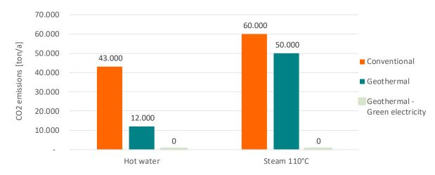
Figure 4: CO2 emissions for geothermal hot water and 110°C steam production.
