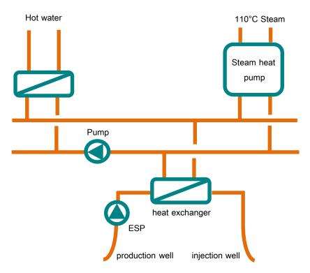
Figure 3: Schematic overview energy concept geothermal energy at Jababeka
