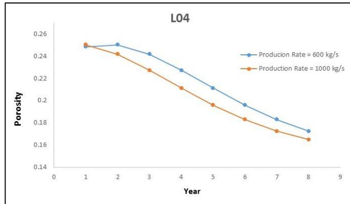
Figure 4.10 Porosity response in reservoir layer.
