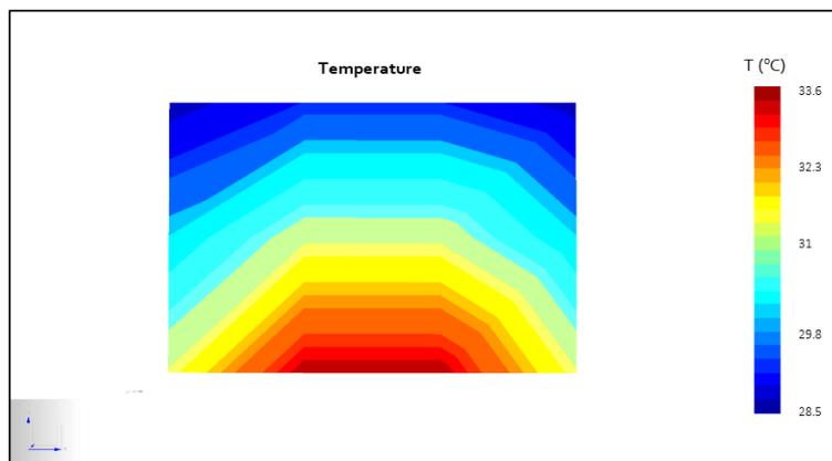
Figure 4.2 Temperature distribution natural state condition of simple synthetic model.
