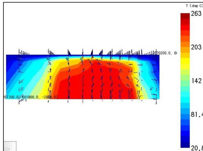
Figure 4.5 Temperature distribution natural state condition of geothermal synthetic model.
