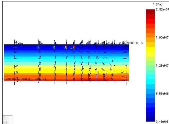
Figure 4.4 Pressure distribution natural state condition of geothermal synthetic model.
