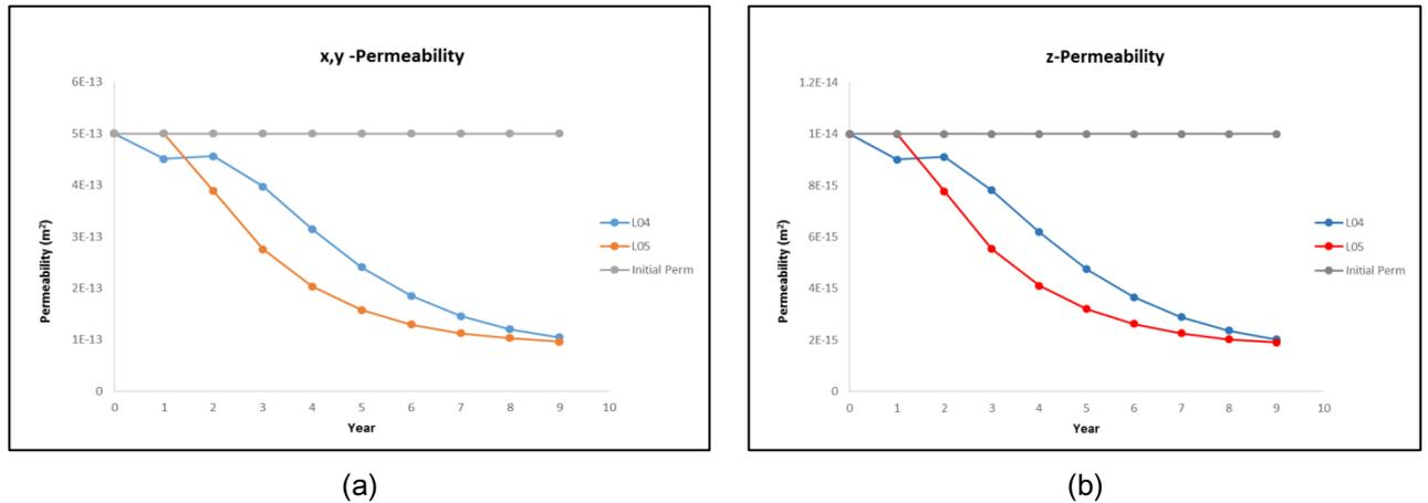
Figure 4.8 Permeability changes in x-y axis (a) and z axis (b).
