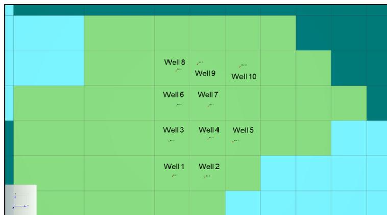
Figure 3.4 Well location in geothermal synthetic model.
