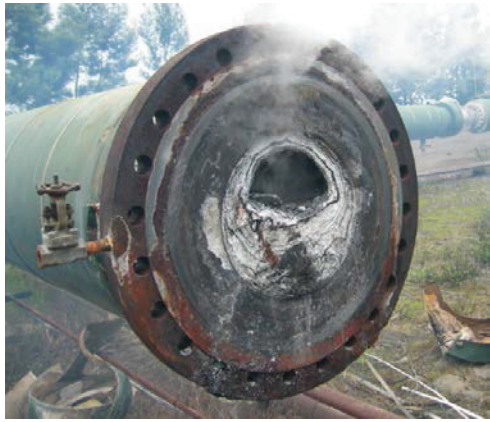
Figure 51 Typical problems found in the fields due to the impurity of geothermal fluid; silica scaling in pipes (left) and erosion on turbine blades (right)
