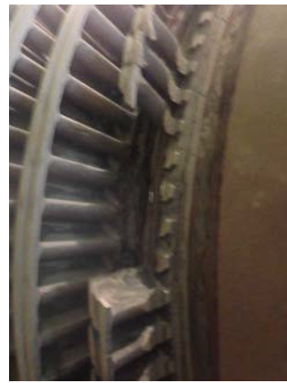
Figure 51 Typical problems found in the fields due to the impurity of geothermal fluid; silica scaling in pipes (left) and erosion on turbine blades (right)
