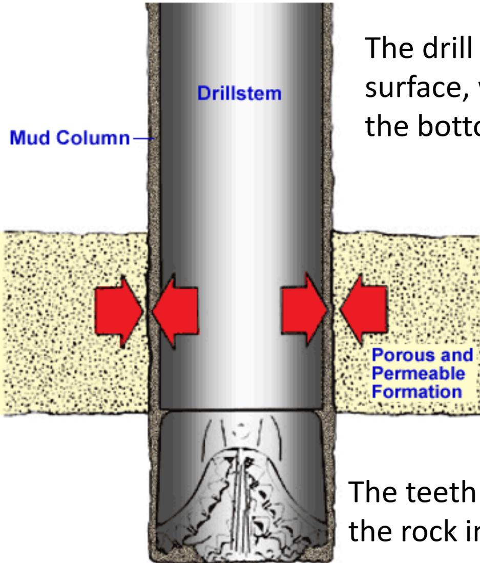
The drill string is turned at surface, which turns the bit at the bottom of the hole.
