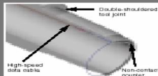
The non-contact coupler fits in a shallow groove inside the secondary shoulder of the eXtreme™ Torque (XT™) connection
