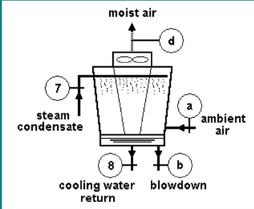
$$\dot{m}_7 h_7 - \dot{m}_8 h_8 = \dot{m}_d h_d - \dot{m}_a h_a + \dot{m}_b h_b$$
