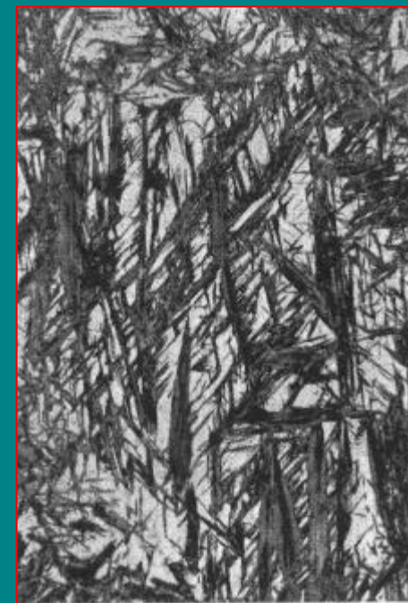
Martensite (needle structure) formed by quick cooling (quenching).
