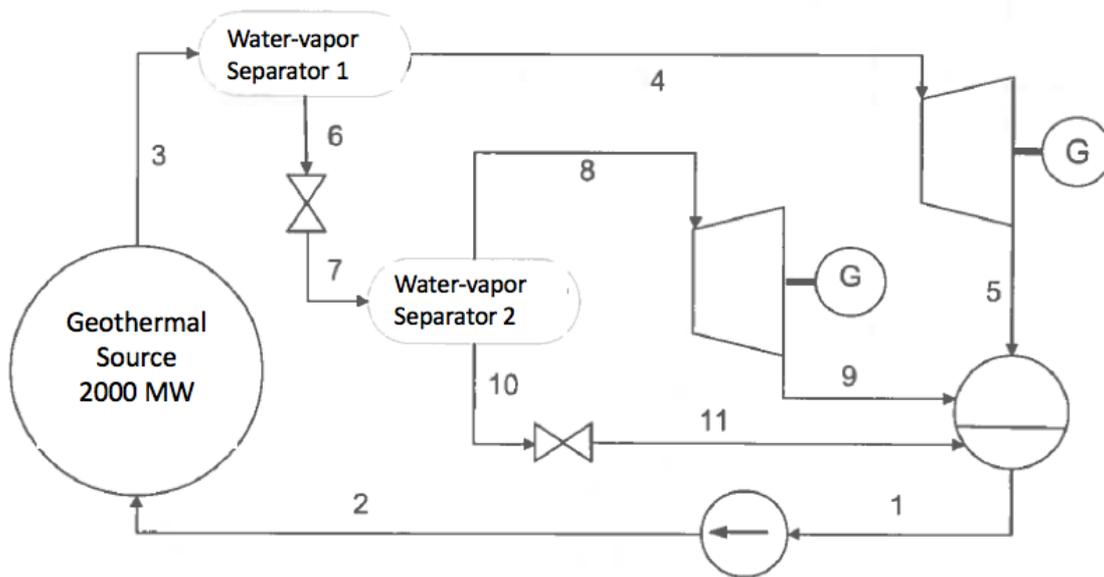
In Iceland electricity is generated in a geothermal power plant with a Rankine cycle with water as a working fluid. The water is originating from a geothermal source and used directly within the cycle. The power on geothermal heat which is extracted from the geothermal source is 2000 MW. Above a schematic picture is given of the geothermal power plant.
