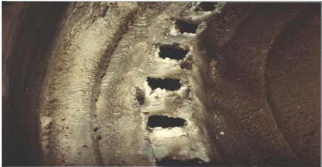
Figure 11: Steam turbine inlet nozzles with intensive scaling.
