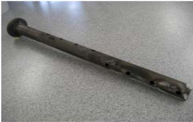
Acid dosing quills before and after brine service at elevated temperatures
