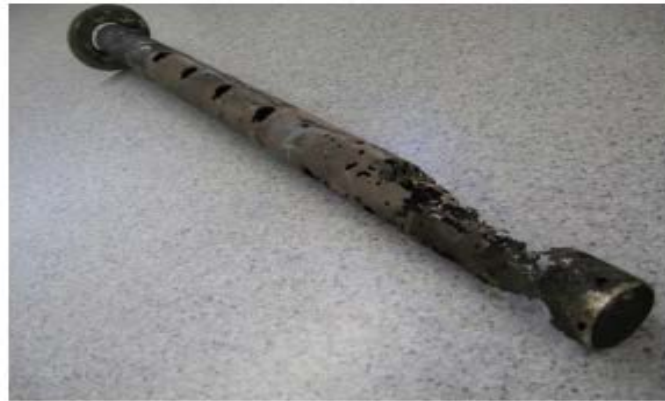
Acid dosing quills before and after brine service at elevated temperatures
