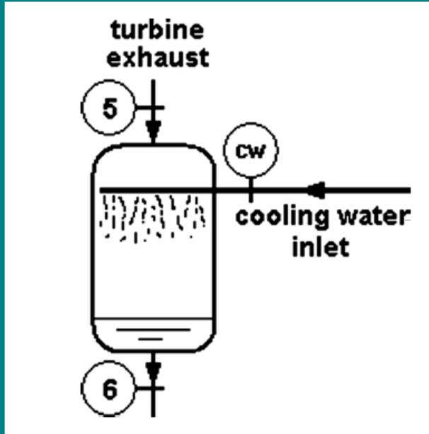
$$\dot{m}_{cw} = x_2 \dot{m}_{total} \left[ \frac{h_5 - h_6}{\bar{c}(T_6 - T_{cw})} \right]$$
