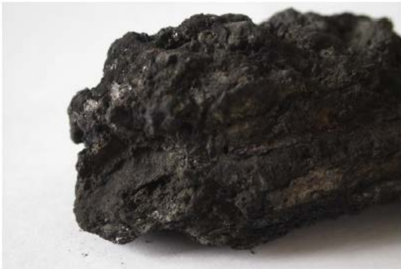
Fig. 3. Corrosion product sample taken from the labyrinth packing.
