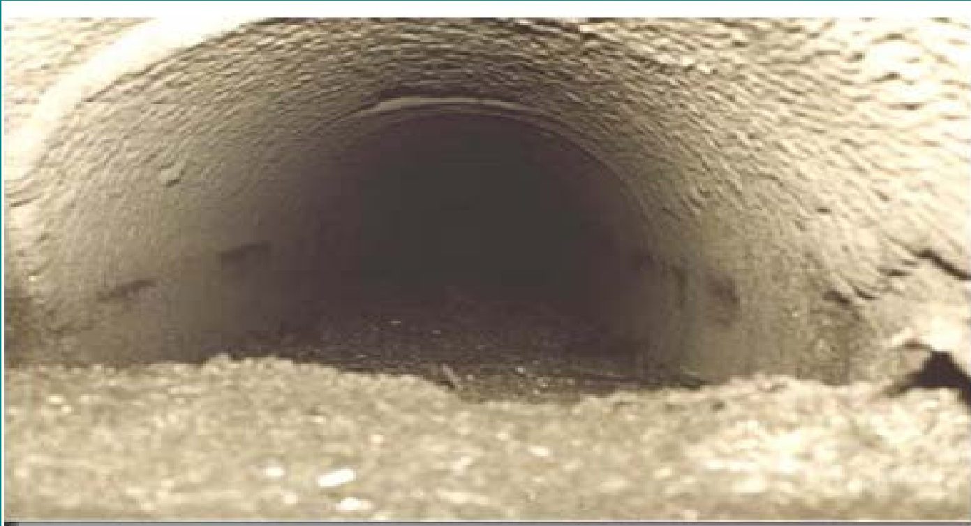
Figure 9: Silica scaling in a 500 mm brine pipe.
