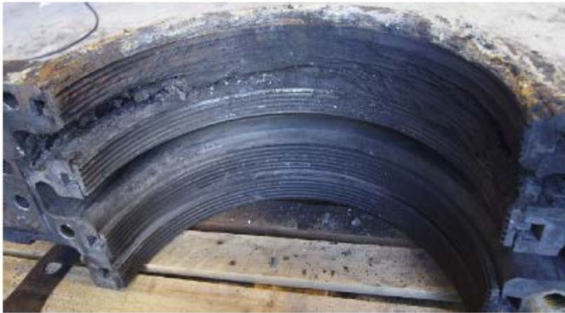
Fig. 2. Corrosion product from the outermost set of labyrinth packing.
