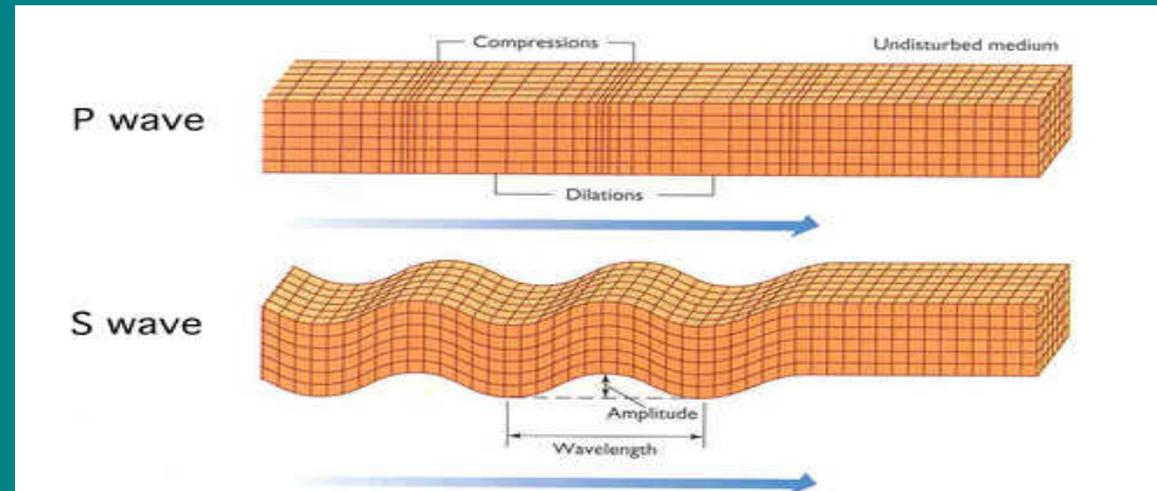
Measurement of Vp, Vs and density
